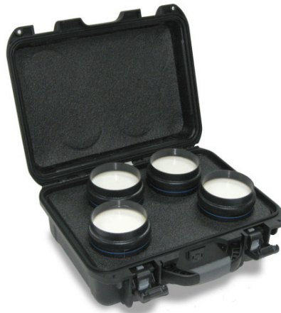
Exhibit 2-7. Shear wave liver fibrosis phantoms
