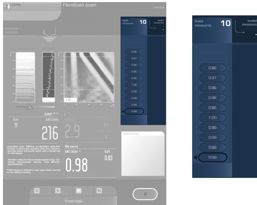
Exhibit 2-18. Counter of valid and invalid measurements
