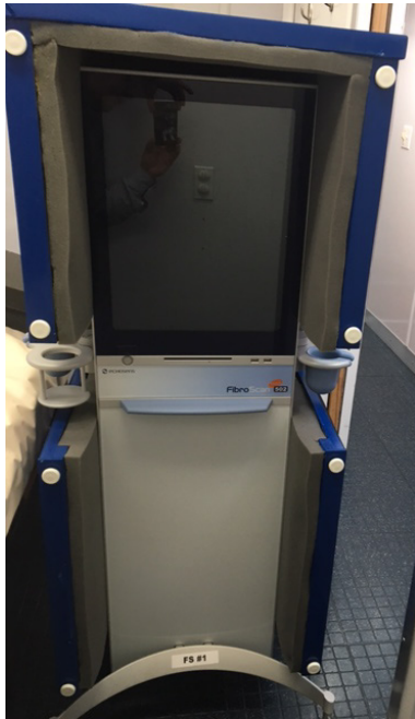
Exhibit 2-42. FS protective box secured to the wall
