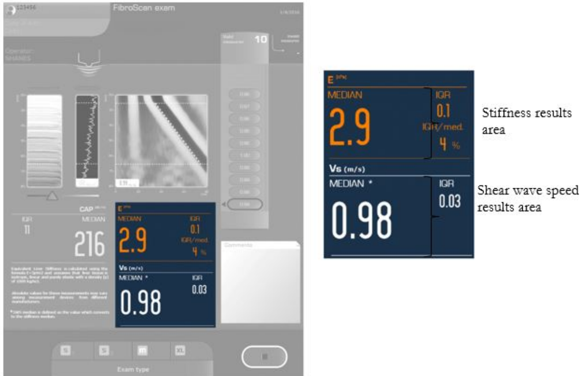
Exhibit 2-20. Stiffness and shear wave speed results area
