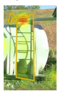
This ladder may not be designed to provide safe access. Mine operators must maintain safe access to all working places and identify where fall protection is needed. Additionally, according to MSHA standards, fixed ladders should project at least three feet above landings, or substantial handholds must be provided above the landings [30 CFR 56/57.11006].
