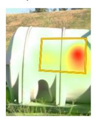
This unlabeled tank may put mineworkers at risk of chemical hazards. According to MSHA standards, mine operators must develop, implement, and maintain a written HazCom program. Operators must identify chemicals, make a hazard determination, ensure that containers of hazardous chemicals have labels, and have and make available a Material Safety Data Sheet (MSDS) for each hazardous chemical used or produced at the mine [30 CFR Part 47].
