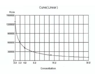
Total T4 concentrations are calculated by using a calibration curve. This method utilizes a four parameter logistic curve with an inverse relationship of measured light produced (RLU) to concentration of total T4 in the serum sample. Serum results are expressed as ug/dL.
