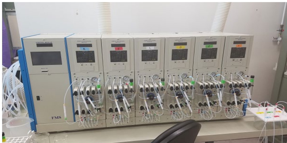
Figure 6.4.1. Fluid Management System (FMS) Power-Prep NG.
