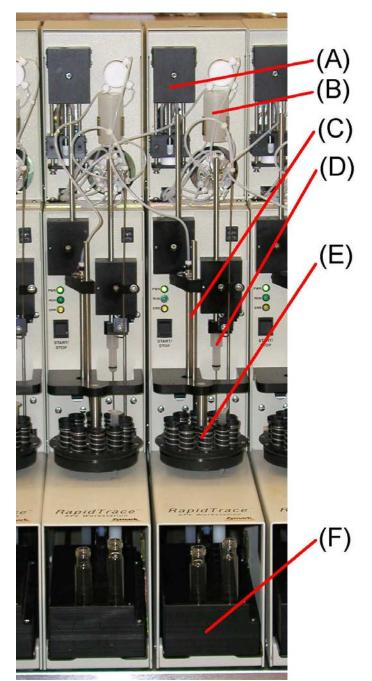
**Figure 2.** Rapid Trace modular SPE work station up to 10 modules controlled by one computer. Instrument includes (A) syringe pump, (B) mixing chamber [not used in current method], (C) plunger, (D) cannula and (F) sample and fraction collection rack.
