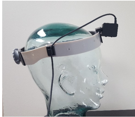
Exhibit 3-55. Headband with accelerometer positioned for vertical testing
