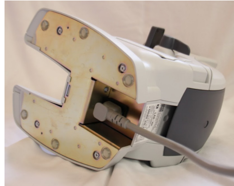
Exhibit 2-3. Power cord connection to lensmeter
