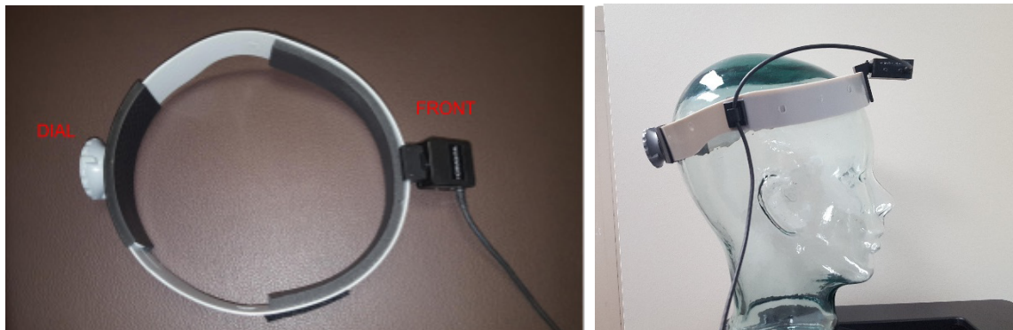
Exhibit 2-17. Headband with accelerometer positioned for horizontal testing
