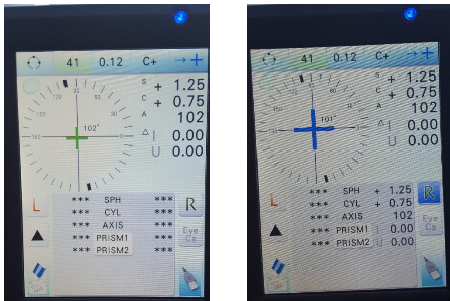
Exhibit 2-14. Finding optical center with the lensmeter
