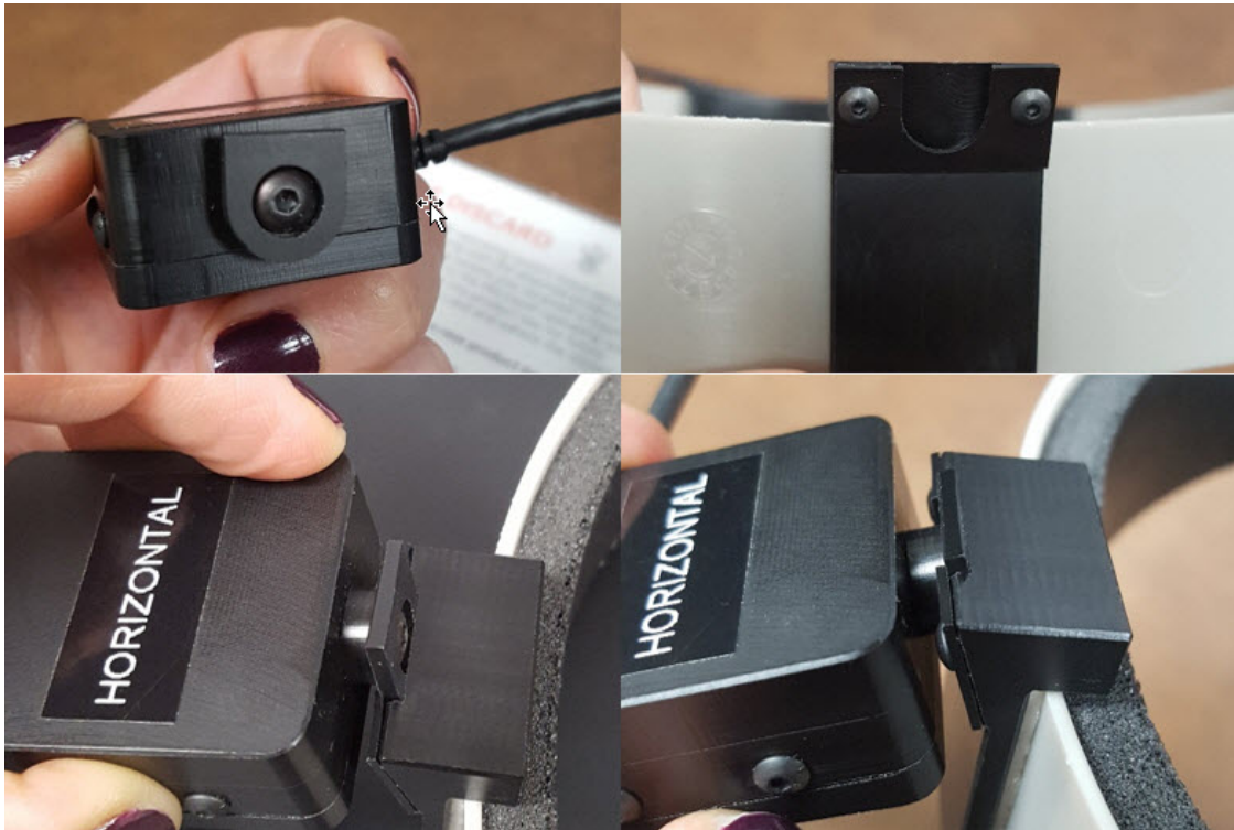
Exhibit 2-7. Attach the motion detector to the headband
