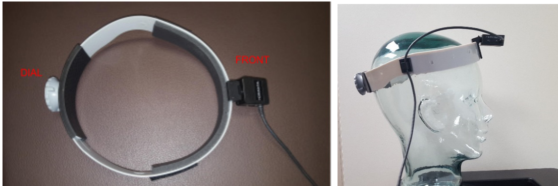
Exhibit 3-52. Headband with accelerometer positioned for horizontal testing
