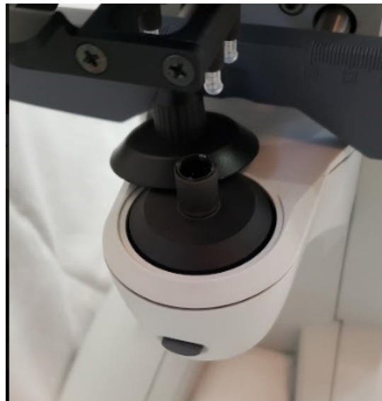
Exhibit 2-12. Lensmeter nose piece lifted for sensor inspection
