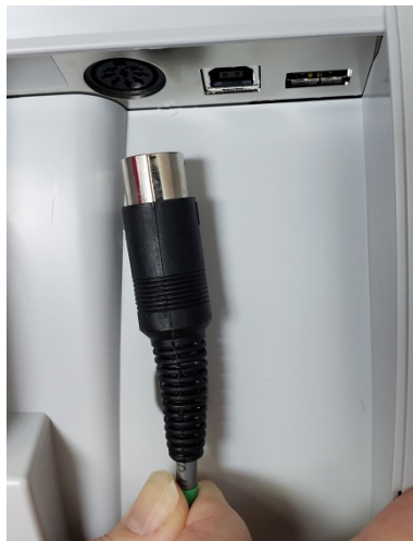
Exhibit 2-4. ISIS computer cable connection to lensmeter
