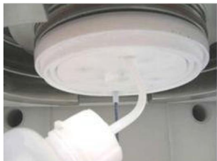
Figure 24 Cleaning procedure, rinsing three channels
