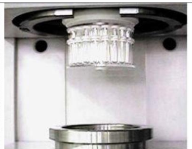
Figure 19 Hanging-up samples with fixed PTFE cover
