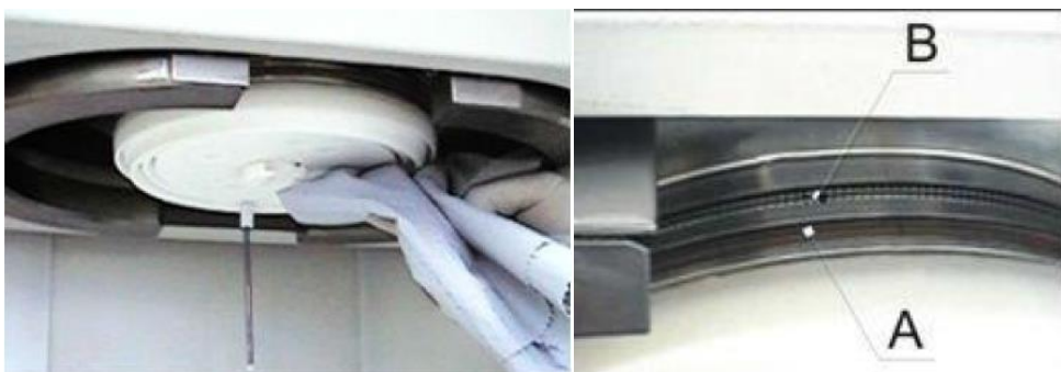
Figure 25 Drying procedure of the microwave digestion vessel
