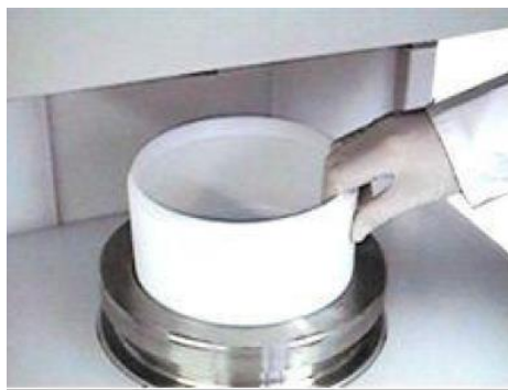
Figure 26 Inserting digestion vessel into pressure chamber
