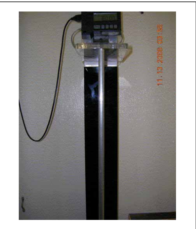
Exhibit 2-8. Stadiometer calibration rod
