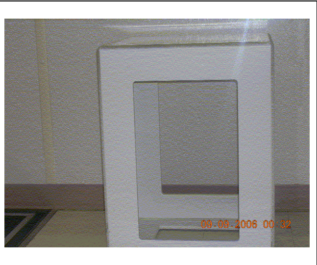
Exhibit 2-8. Stadiometer calibration rod
