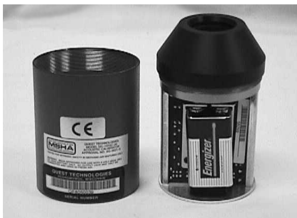
Changing the Battery in the Calibrator
