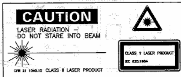
Figure 2-3. Laser warning label
