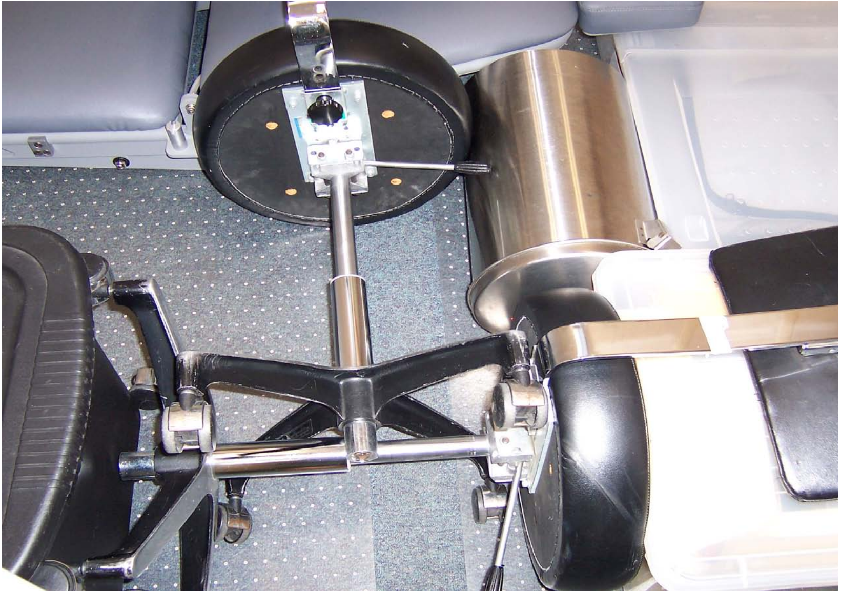
FLOOR STORAGE: Close-up showing placement of stools to minimize shifting in transport. Stools are tipped on side with stool backs extended.
