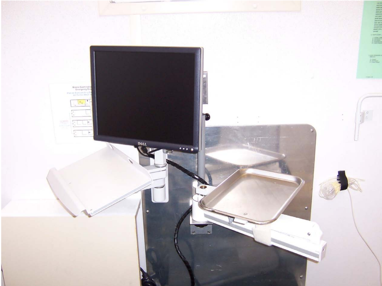
COMPUTER STAND AND INSTRUMENT TRAY: Fold articulating arms on computer wall mount and light holder/instrument tray. Secure with Velcro or bungee cords.
