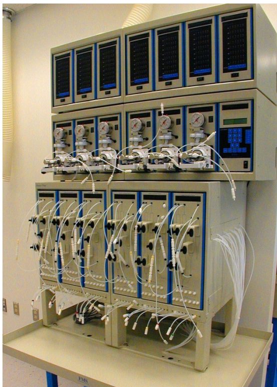
Figure 1. Fluid Management System (FMS) Power-Prep/6.
