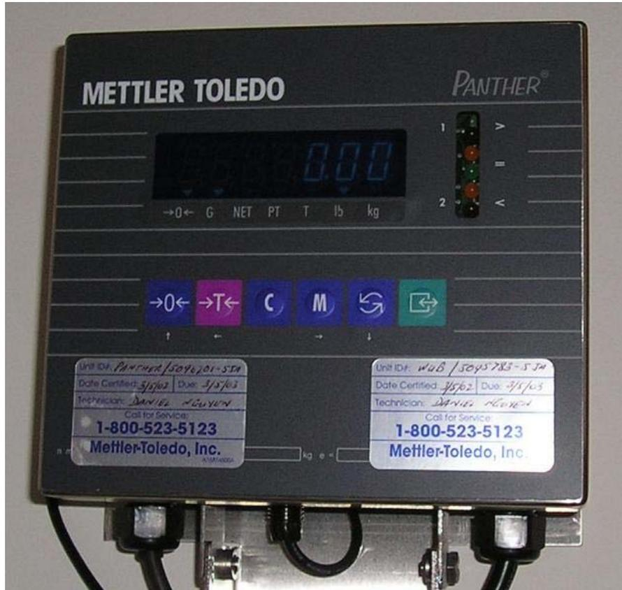
The device contains a row of six buttons. The second button from the right has two arrows that toggle the display from pound to kilogram units. Above this button is an upside down triangle that points to either the “kg” or “lb” display label. Keep the display toggled to kg at all times.
