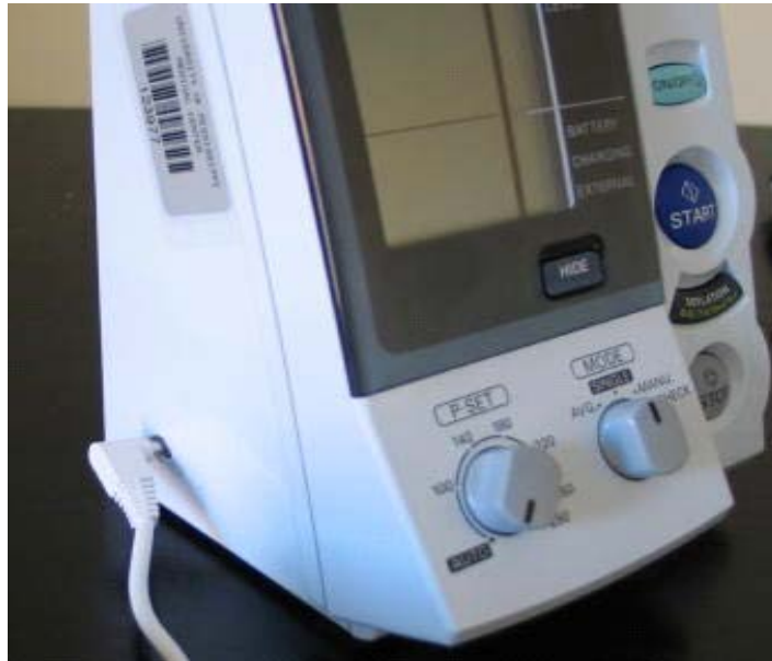
Exhibit 4-2. The Omron showing plugged in DC jack
