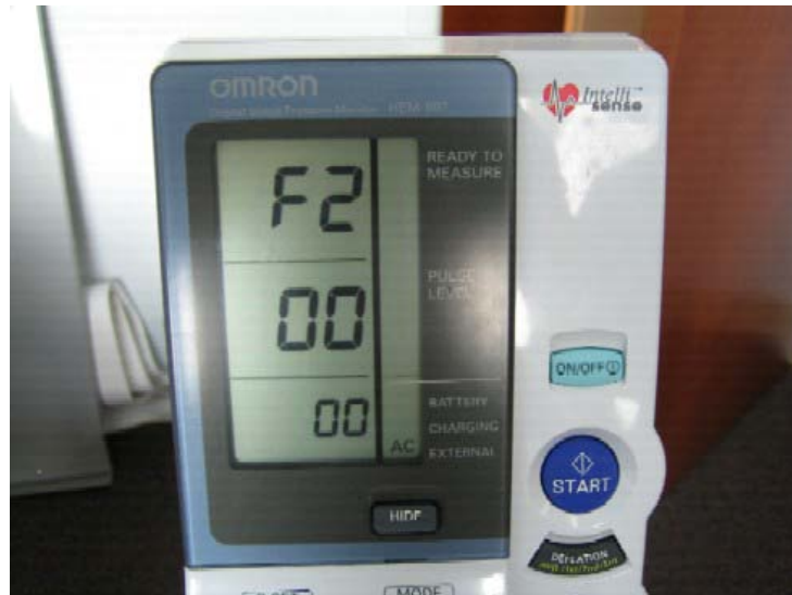
Exhibit 4-5. The F2 function setting to 0 seconds waiting time until the first measurement
