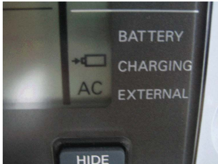
Exhibit 4-3. AC sign visible in lower window
