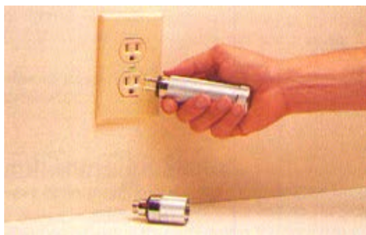
Figure 2-28. Charging the otoscope (NOTE: It is not necessary to remove the head of the scope in order to charge the handle.)
