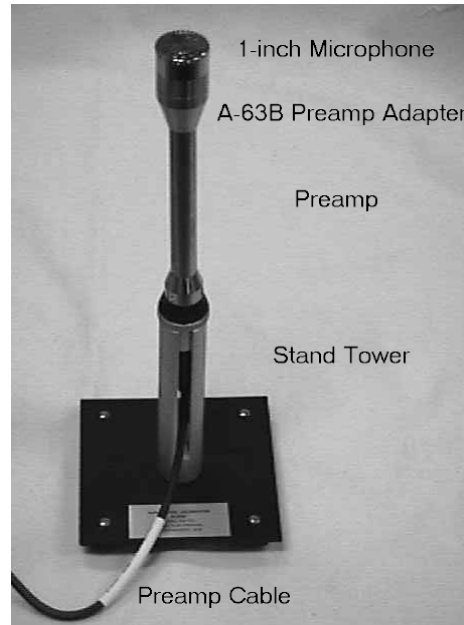
Figure 2-18. Assembled calibration tower
