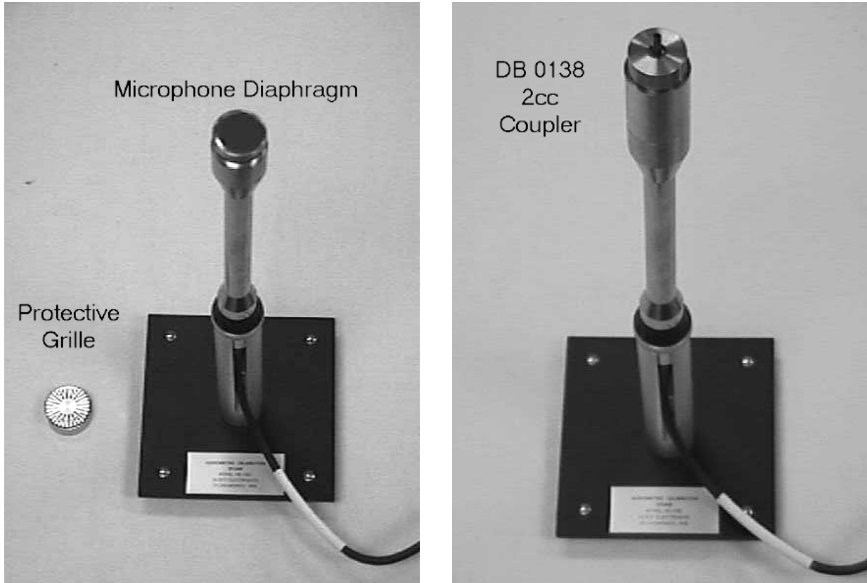
Figure 2-21. Microphone with grille removed (left) and coupler attached (right)
