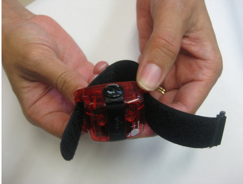
Exhibit 3-11. Threading the wrist strap through the PAM
