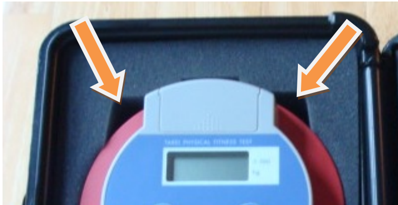
Figure 2-8. Storing dynamometer batteries
