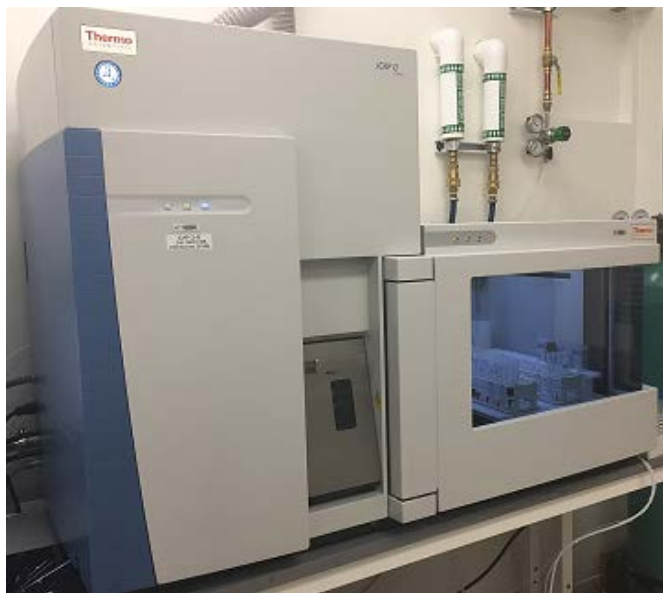
Figure 6-1: iCAP Q ICP-MS with integrated autosampler housing
