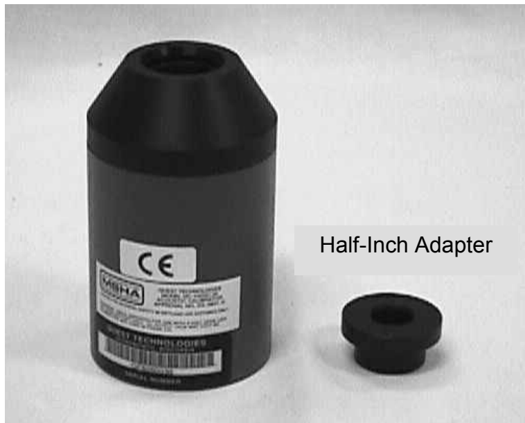
Figure 2-10. Quest Model QC-20 calibrator with adapter
