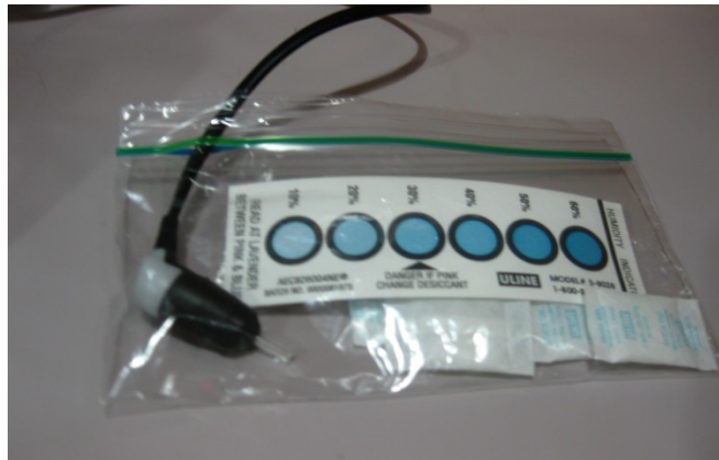
Figure 2-47. Titan probe tip storage
