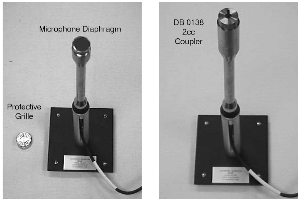
Figure 2-26. Microphone with grille removed (left) and coupler attached (right)
