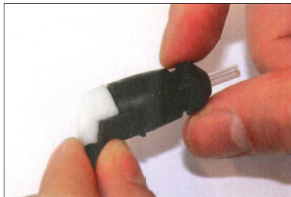
Figure 2-36. Unscrew the probe cap from the probe tip
