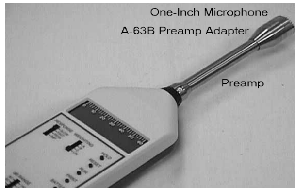
Figure 2-31. Sound level meter connected to preamp and microphone
