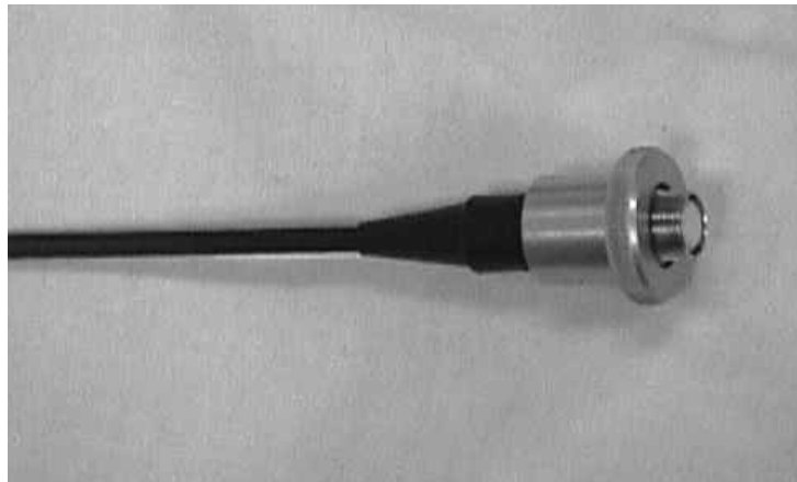
Figure 2-22. Assembly of preamp cable
