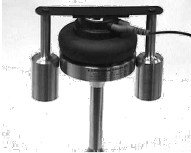
Figure 2-27. Earphone mounted on coupler
