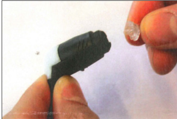
Figure 2-37. Pull the probe tip directly off the probe
