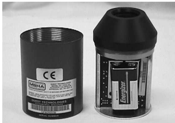
Figure 2-33. Changing battery in the calibrator
