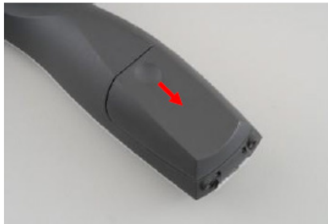
Figure 2-42. Removing the battery cover from the Titan handheld unit
