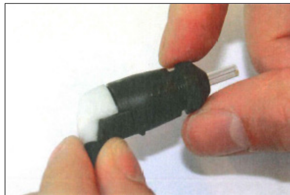
Figure 2-40. Screw the cap back onto the probe
