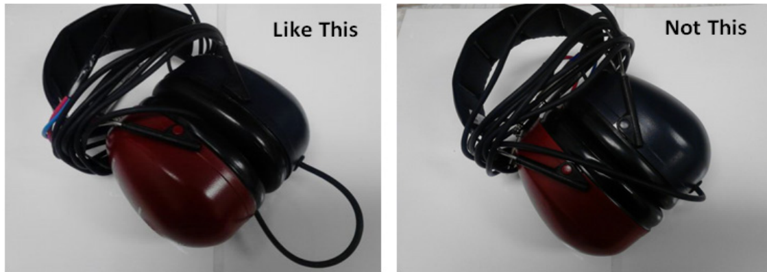
Figure 2-49. Correct and incorrect ways to protect cables at attachment points to equipment
