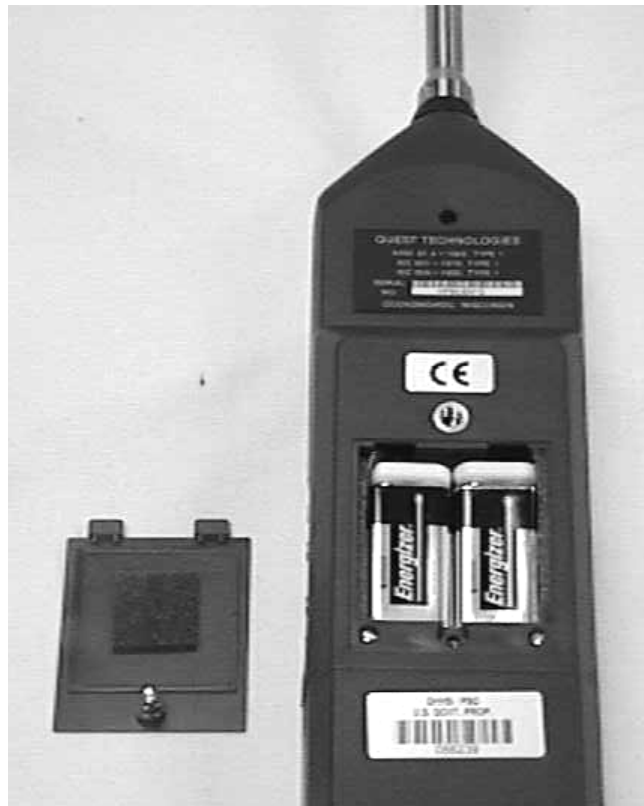
Figure 2-32. Changing batteries in sound level meter
