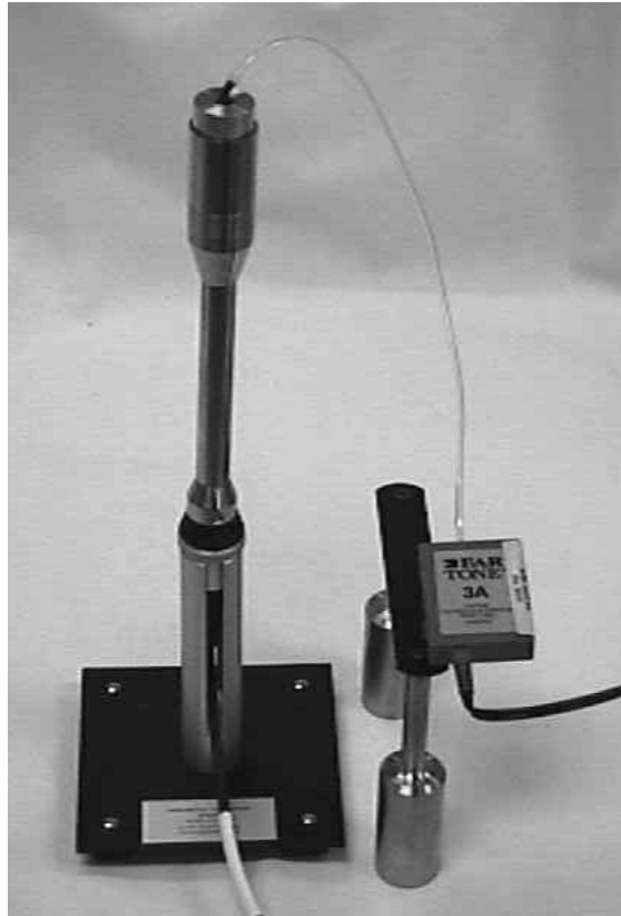
Figure 2-28. Insert earphones in coupler
