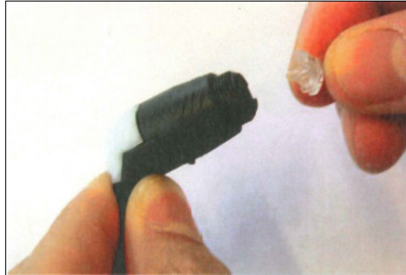
Figure 2-39. Snap the tip back onto the probe
