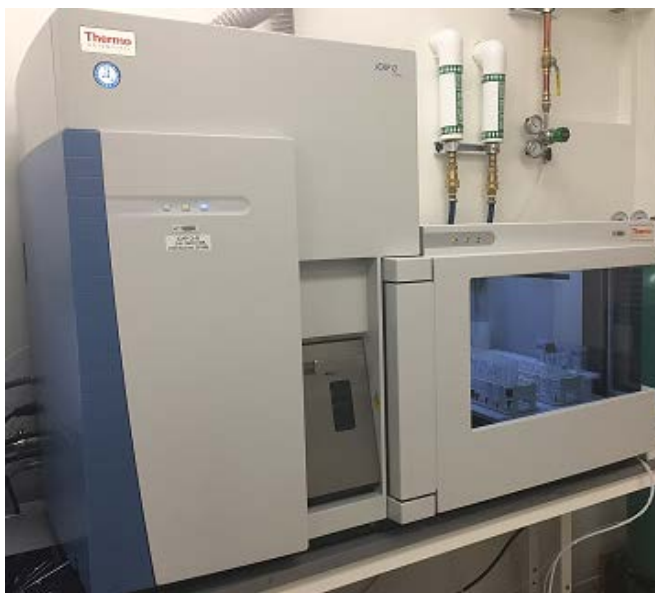
Figure 6-1: iCAP Q ICP-MS with integrated autosampler housing
