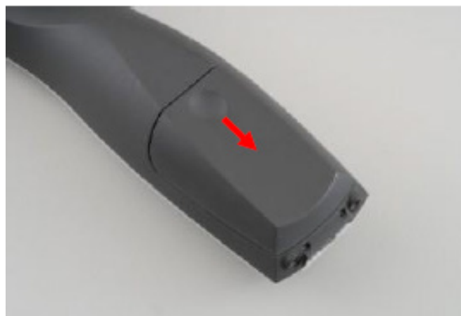
Exhibit 2-65. Removing the battery cover from the Titan handheld unit
