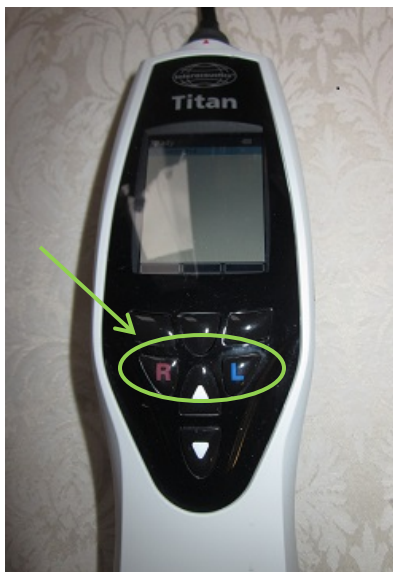
Exhibit 3-15. R and L buttons on the Titan handheld unit
