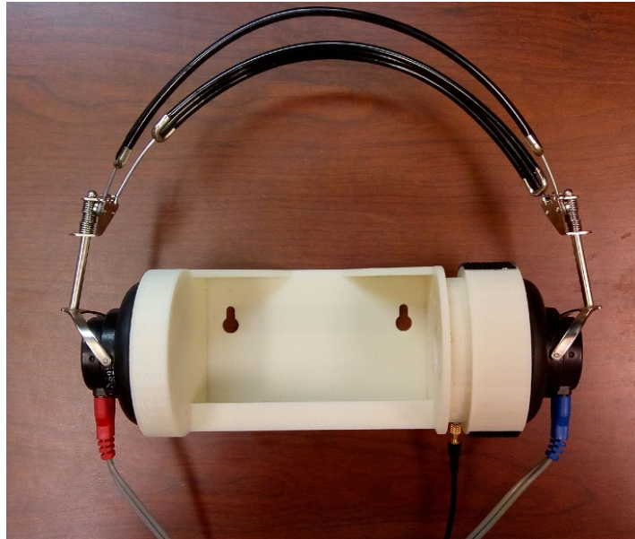
Exhibit 2-39. Standard headphones mounted to calibration fixture
