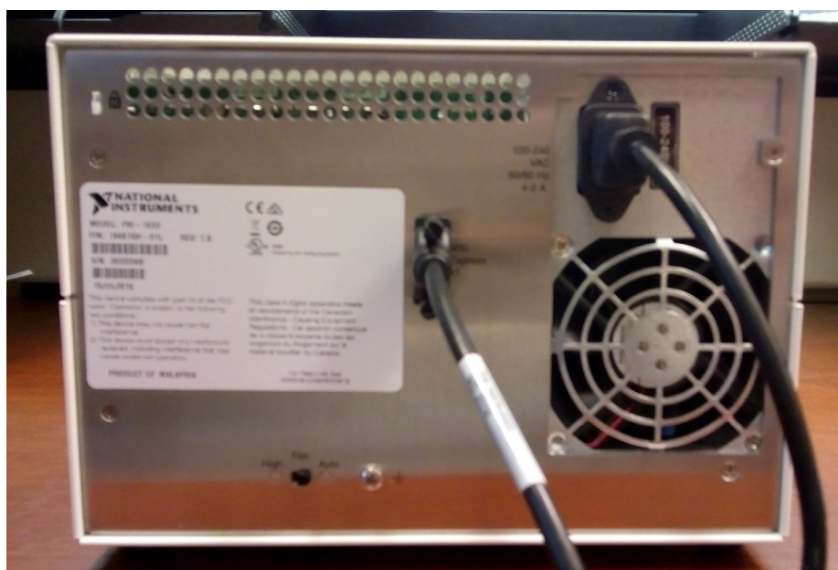
Exhibit C-1. Connections on the back of the ART chassis
