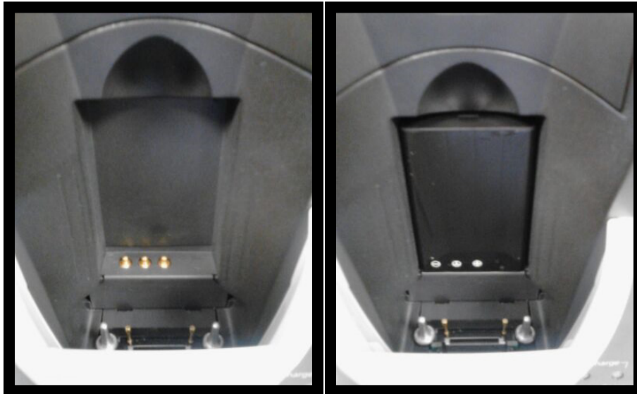
Exhibit 2-14. Spare Titan battery in cradle holder
