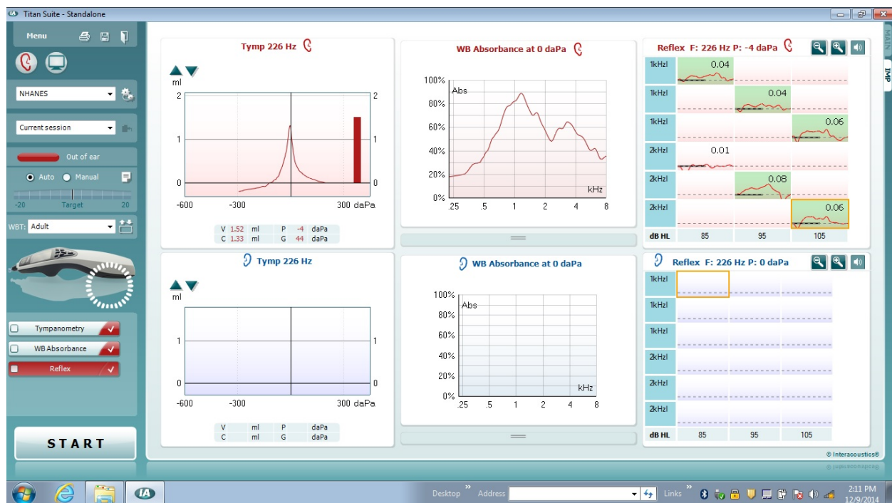
Exhibit 3-19. Sample Titan Suite screen showing a completed test in the right ear
