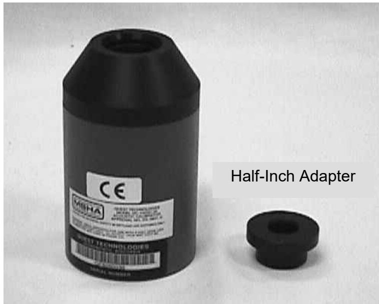
Exhibit 2-9. Quest Model QC-20 calibrator with adapter
