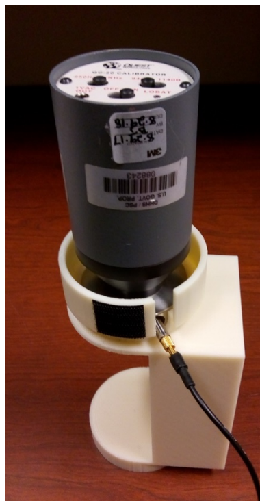
Exhibit 2-31. Calibrator on the coupler base
