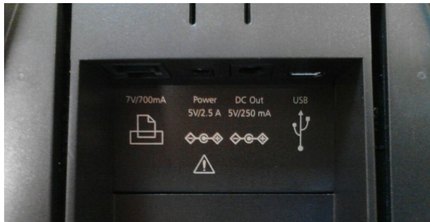
Exhibit 2-11. Charging cradle connections
