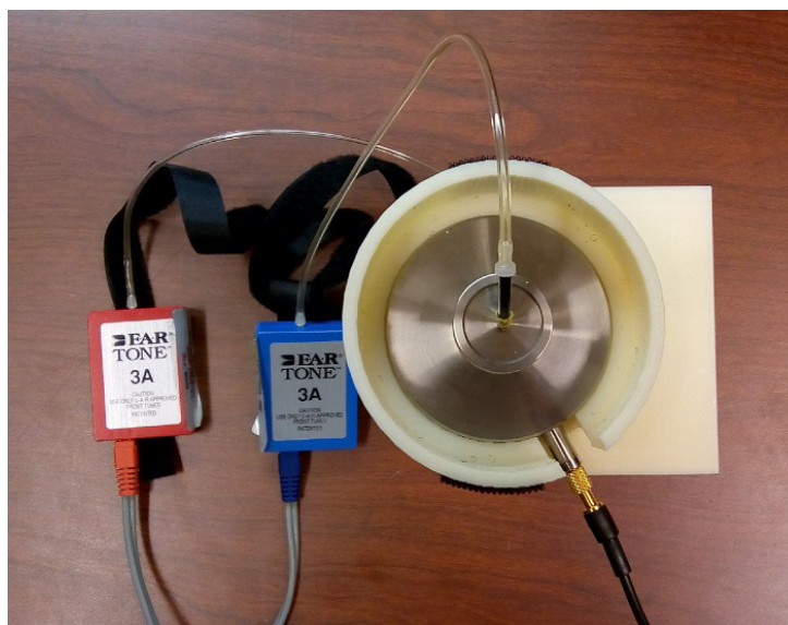
Exhibit 2-40. Insert earphones mounted to calibration fixture
