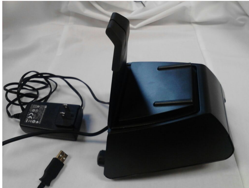
Exhibit 2-12. Cradle back plate in position, covering the USB and power cord connections
