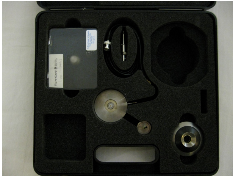
Exhibit 2-78. Calibration case with standard and insert earphone couplers
