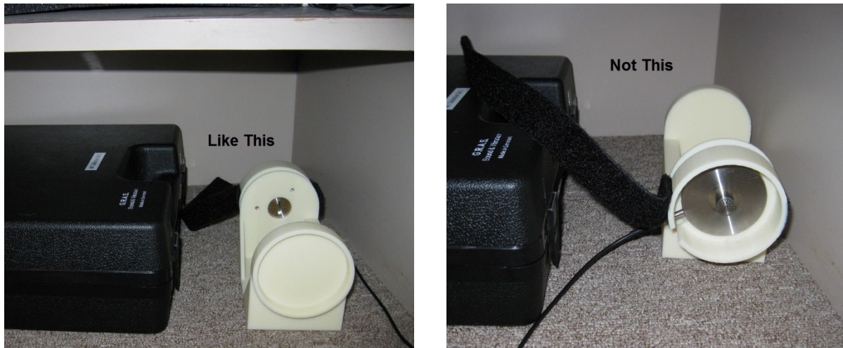
Exhibit 2-21. Correct placement of the calibration fixture when storing it beneath the table inside the sound booth
