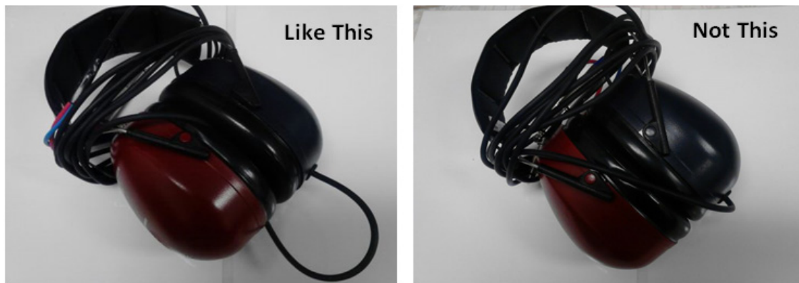
Exhibit 2-73. Correct and incorrect ways to protect cables at attachment points to equipment
