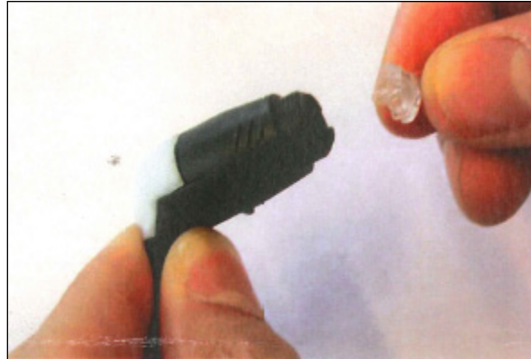
Exhibit 2-60. Pull the probe tip directly off the probe
