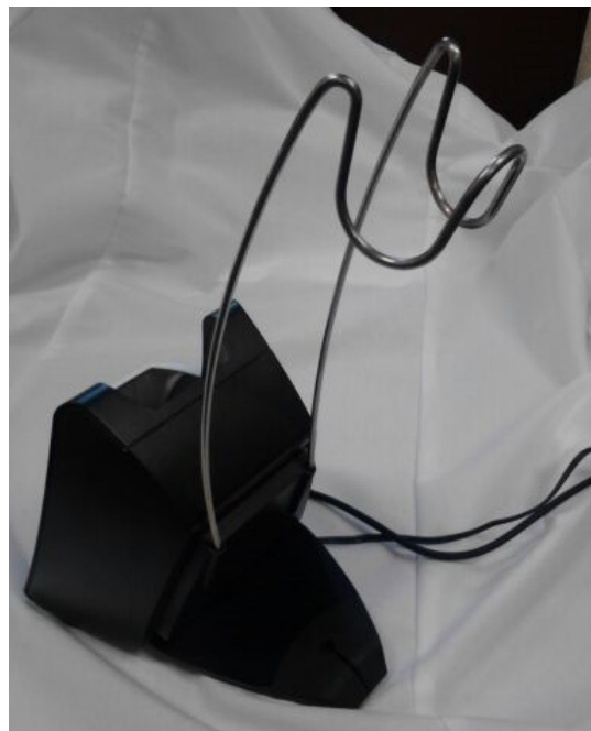
Exhibit 2-13. Steel cable holder inserted into back plate
