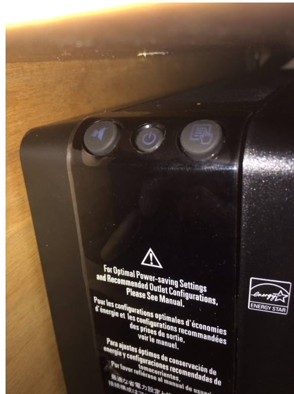
Exhibit 9-3. Photo showing shutdown button
