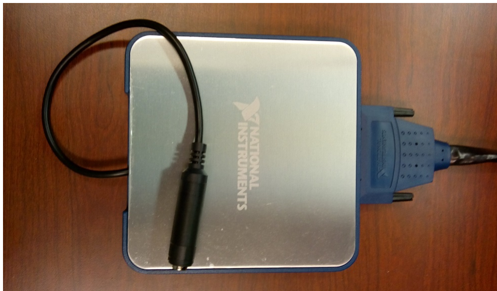
Exhibit C-7. Ridiculously massive response switch cable attached to the National Instruments response switch box
