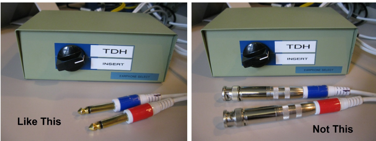
Exhibit C-11. Correct (left) and incorrect (right) point of disconnection between the headphone selector box cables and the ART headphone cables
