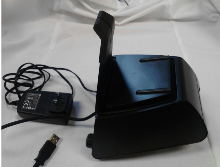
Exhibit 2-14. Cradle back plate in position, covering the USB and power cord connections
