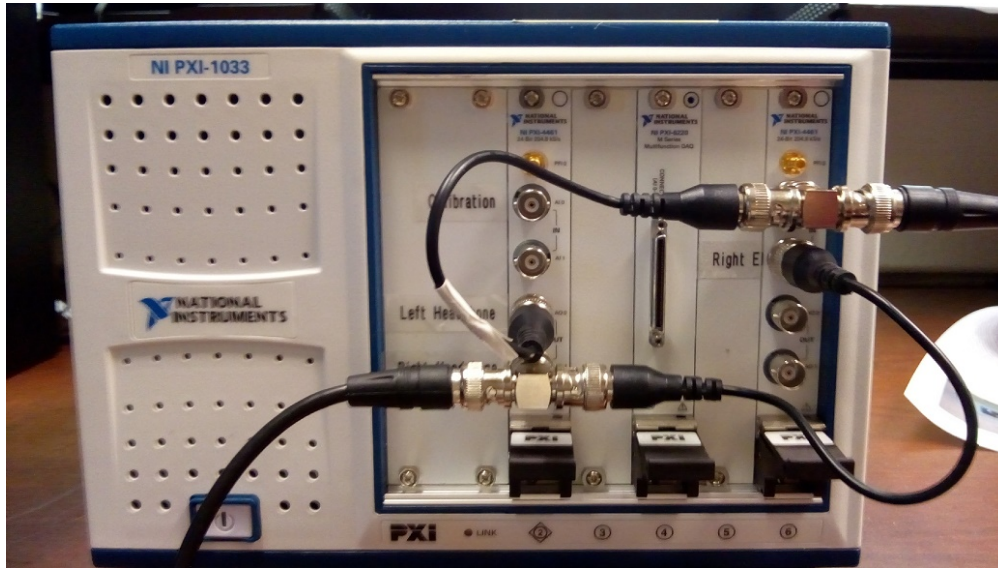
Exhibit C-5. Right BNC headphone assembly attached to the front of the chassis
