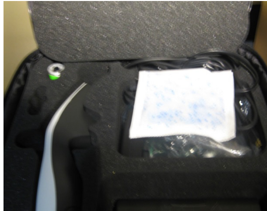
Exhibit 2-72. Probe packed near desiccant pillows
