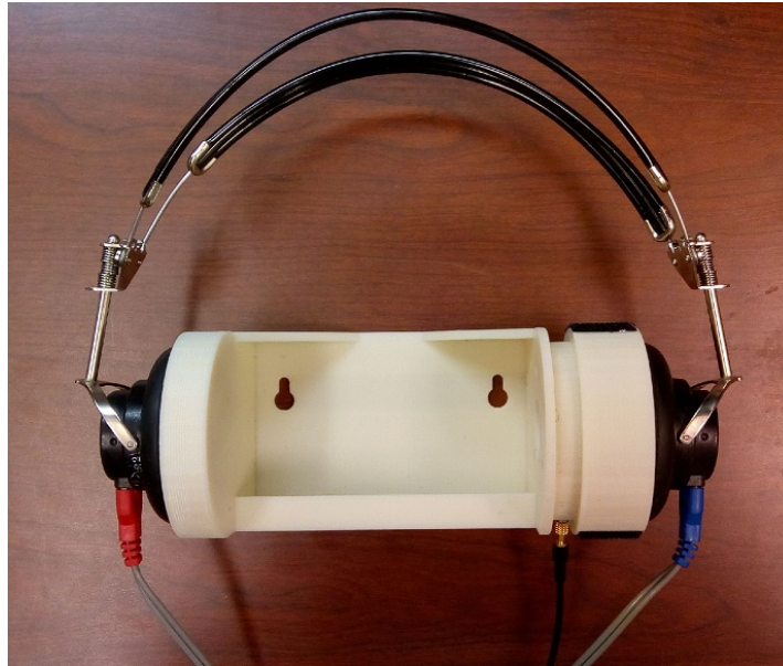
Exhibit 2-40. Standard headphones mounted to calibration fixture
