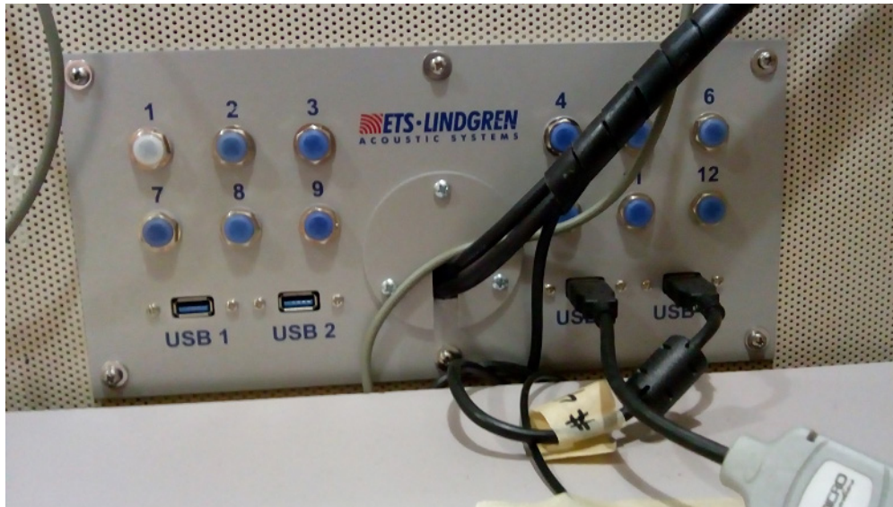
Exhibit 2-81. Jack panel and work station inside the audiometric booth prepared for transport
