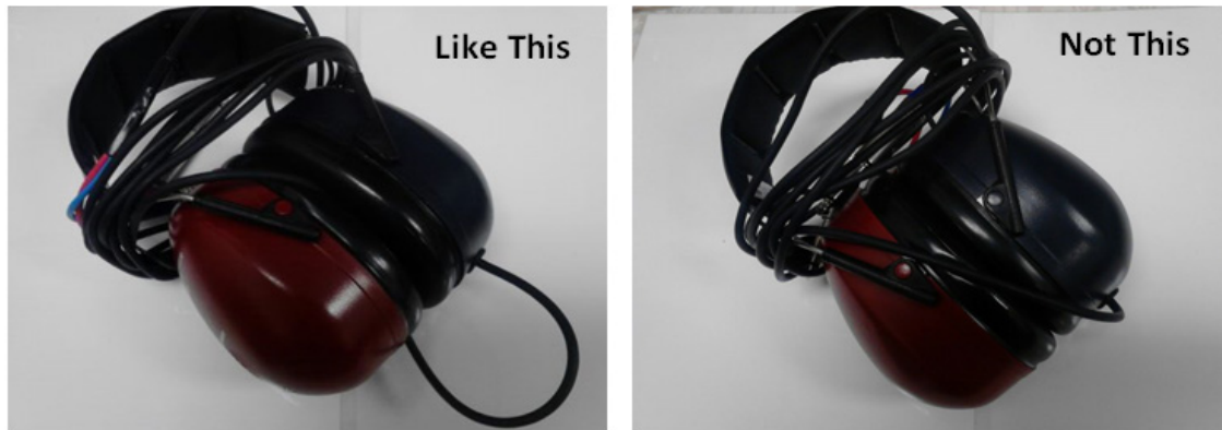
Exhibit 2-77. Correct and incorrect ways to protect cables at attachment points to equipment
