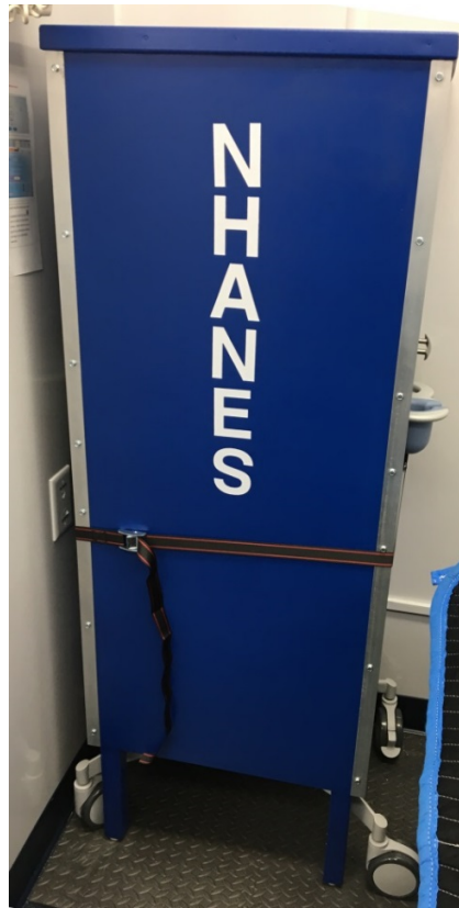
Exhibit 2-42. FS protective box secured to the wall
