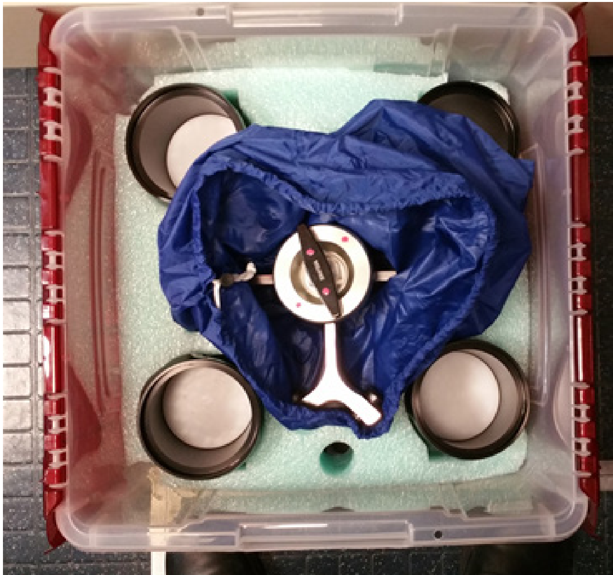
Exhibit 7-17. Packing rotors in plastic bin (1)
