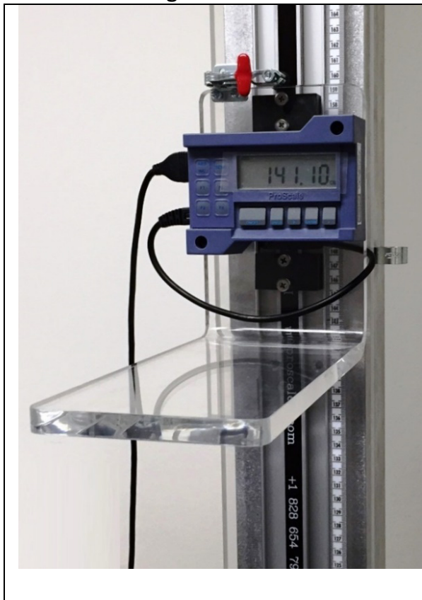
Exhibit 2-6. Stadiometer headpiece and digital measurement device
