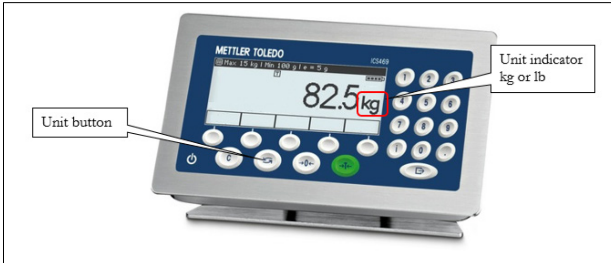
Exhibit 5-6. Digital scale measurement device
