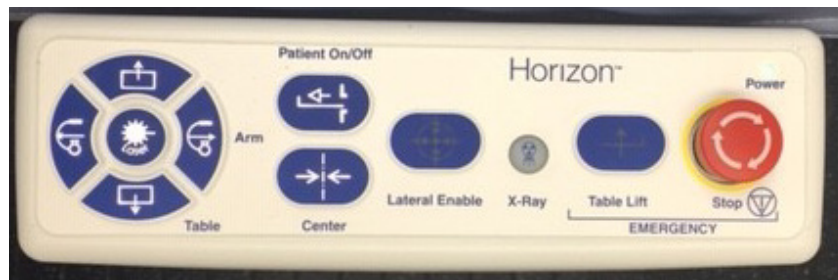
Figure 3-2. Horizon A Table instrument control panel
