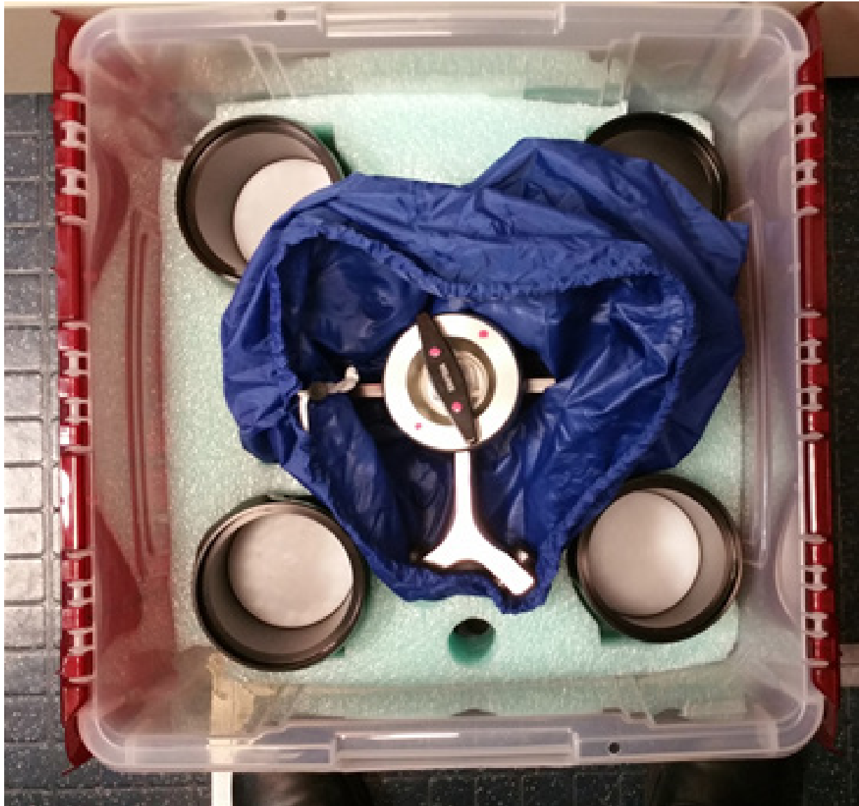
Exhibit 10-4. Proper packaging of centrifuge rotors
