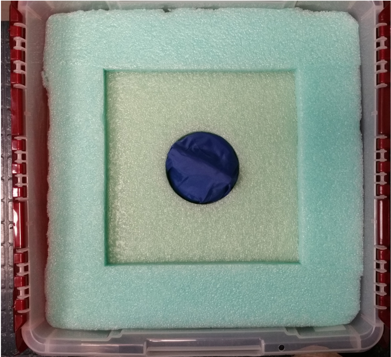
Exhibit 10-5. Proper packaging of centrifuge rotors (2)
